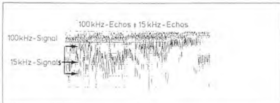
Figure E-7: Echo sounding penetration [De Brauwer, 2005]
