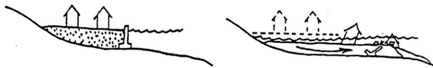
Fig. 4-3 a typical example of ground horizontal displacement as a result of lateral dispersion due to the occurrence of liquefaction behind seawall
