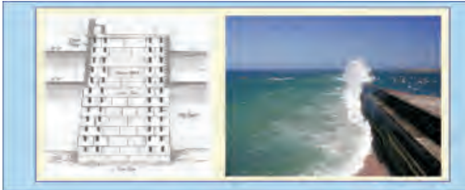
Fig. 7.13: Battered walls: typical cross-section (left), and Admiralty Breakwater, Alderney Channel Islands (right, courtesy G. MÜLLER)
