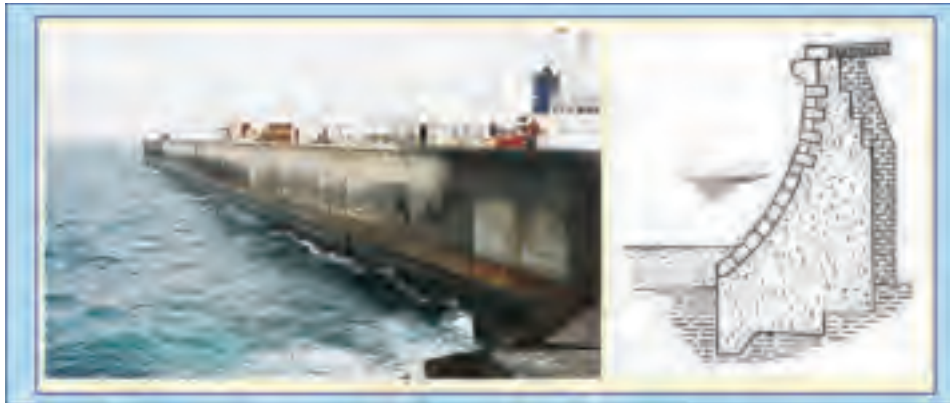
Fig. 7.17: An example of a modern, large vertical breakwater with wave return wall (left) and cross-section of an older seawall with recurve (right)
