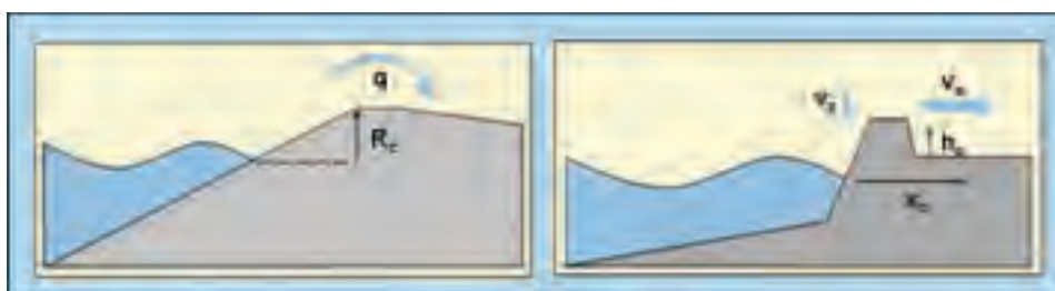
Fig. 3.1: Overtopping on embankment and promenade seawalls
