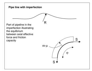
Figure 4-2 Simplified calculation of required pullback forces
