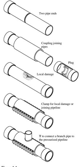
Figure 1-1 Typical installed fittings for repair
