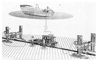
Figure 1-3 Typical support systems for a pipeline repair
